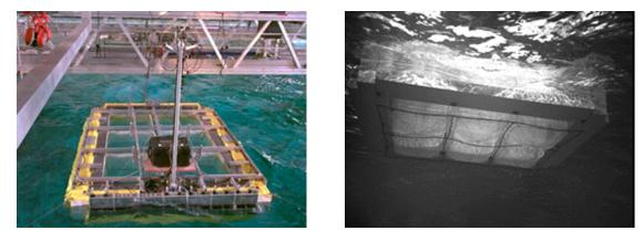
Various designs for the platform have been studied by means of computational analysis to determine their behavior under a wide range of sea conditions. The selected configuration was planned to be studied also via experimental testing. A 1:40 scale model of the selected design was then built and tested in a wave tank trial at the Ecole Centrale de Nantes (FR), in order to validate the computer model assumptions.
